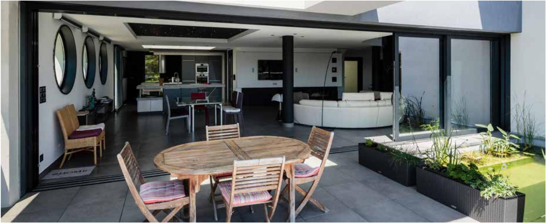
This built in design enables each of the door leaves to be fully retracted and concealed within the walls of the surrounding structure, creating an impressive 9 m wide opening in the building.
